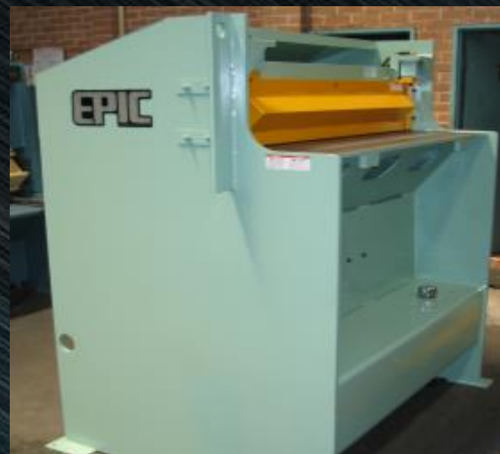
UD6 Guillotine – 6.5mm mild steel capacity
