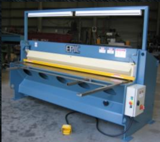
UD4 Guillotine – 4mm Mild steel capacity with Overhead lighting
